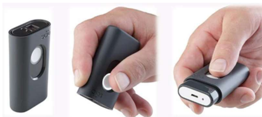
Figure 12: Pocket near-infrared spectrometer to predict beef marbling
