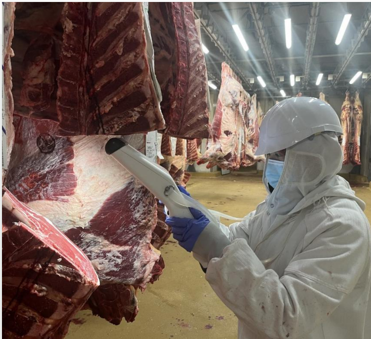
Fig 3: Grading of carcasses for marbling using the Q-FOM™ Beef handheld camera
